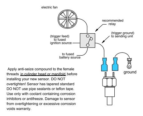
NOTE: An American Autowire relay kit is recommended for this application. We manufacture high quality fan relay kits.
